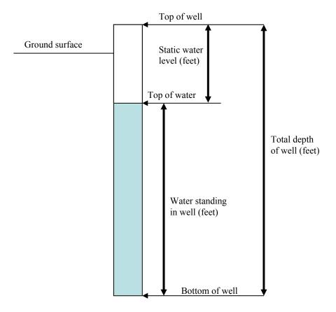
Figure 1. A generalized diagram of a water well.
